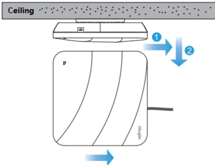
(2) If the AP is installed on the wall, hold the AP with your hands and push it upward and away from the bracket in the LAN port direction.
