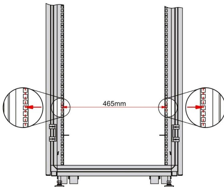
(3) The distance between the square hole strip on the rack column and the outer side of the front cabinet door is greater than 180 mm (7.09 in.) and the thickness of the front cabinet door is smaller than 25 mm (0.98 in.). Therefore, the available space is greater than 155 mm (6.10 in.). The cabinet depth (the distance between the front and rear doors) is greater than 1000 mm (39.37 in.).
