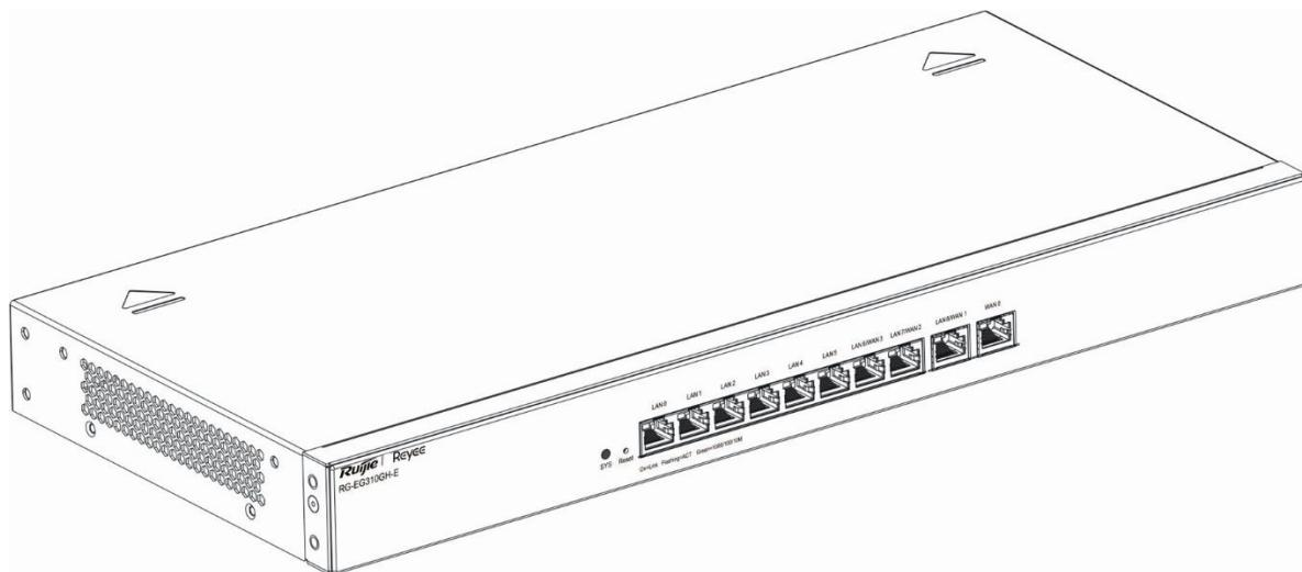
**Figure 1-5 Front Panel of an RG-EG310GH-E Router**
