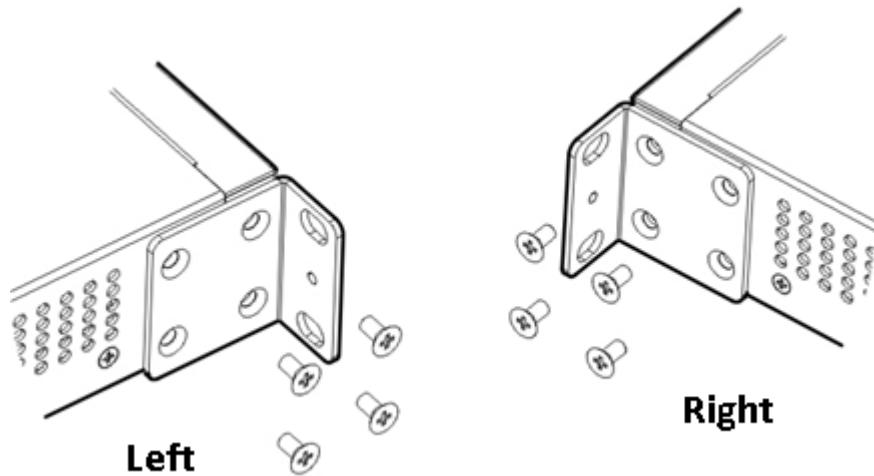
Step 2: Use the supplied M6 screws and cage nuts to securely attach the mounting brackets to the rack, as shown in [Figure 3-2](#) and [Figure 3-3](#).
