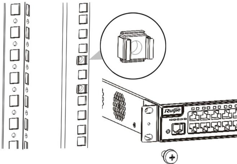
**Figure 3-3 Attaching the Brackets to the Rack**
