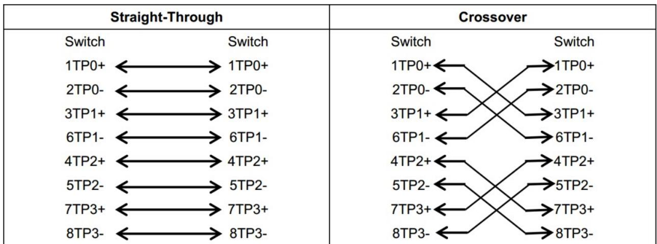
In addition to the preceding cables, the 100BASE-TX/10BASE-T can also use 100-ohm Category-3, Category-4, and Category-5 cables for 10 Mbps, and 100-ohm Category-5 cables for 100 Mbps, both of which can be up to 100 m. [Figure 6-2](#) shows the pinouts of the 100BASE-TX/10BASE-T.
