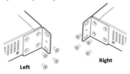
Step 2: Use the supplied M6 screws and cage nuts to securely attach the mounting brackets to the rack, as shown in Figure 3-2 and Figure 3-3.
