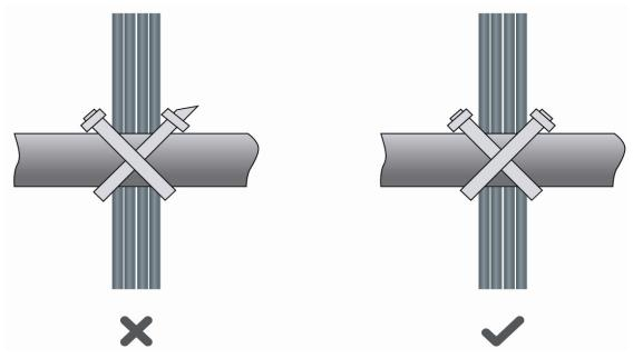
• If cables are to be bent, bind them first but do not tie cable ties within the bend to avoid stress on the cables, which may cause the wires inside to break, as shown in Figure D-3.
