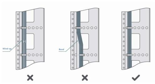
Route and bundle power, signal, ground cables separately. When the cables are close to each other, cross them. When power cables are parallel to signal cables, the distance between them must be 30 mm (1.18 in.).
