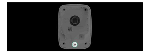
7. Loosen the screws with a PH1 cross-head screwdriver.
