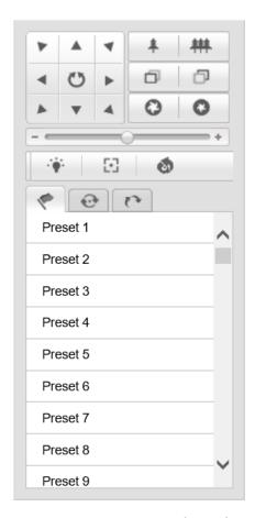
Figure 4-1 PTZ Control Panel
