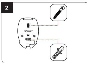
Insert 2 plastic anchors in the holes. Fit the mounting plate of the GALEO and screw it on the wall.
