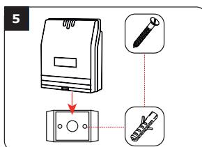
Insert 2 plastic anchors in the holes. Fit the mounting plate of the electronics box and screw it on the wall. Slide the box from top to bottom on the bracket.
