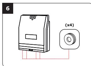
Insert the cable into the remote electronics box and wire the cable to the terminals. Do not forget to install the varistor on the lock (Refer to page 5 "Notes and Recommendations").
