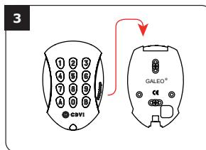
Insert the cable into the holes of the back plate. Then mount the keypad on the back plate, first placing the top in the hooks and then the bottom.
