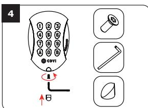
Fasten the GALEO keypad to the back plate by using the supplied (M4x10) Torx® screw and T20 Torx® spanner hardware. Place the screw cap at the bottom of the keypad.
