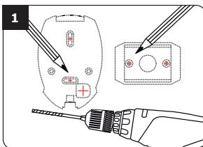
Verify the distance between the GALEO keypad and its remote electronics (Refer to page 5 "Notes and Recommendations"). Place the back plate of the GALEO on the wall and the bracket of the remote electronics box, then mark the hole location with a pen. Then drill the 2 mounting holes (drill bit Ø 5 mm and 35 mm hole depth) and the hole wiring access.
