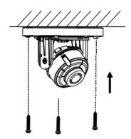
Figure 4, Mounting Base Attachment
