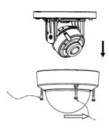
Figure 3, Dome Cover Removal
