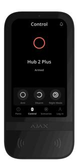
If Group Mode is enabled, users see the security mode of each group separately. The group is armed if its button outline is white and marked with the  $\bigcirc$  icon. The group is disarmed if its button outline is grey and marked with the  $\bigcirc$  icon.
