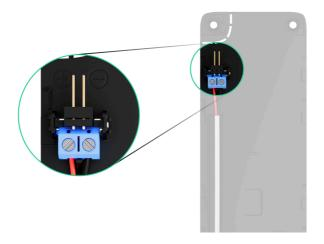
**4.** Route the cable in the cable channel. An example of how to output the cable from the bottom of the keypad:
