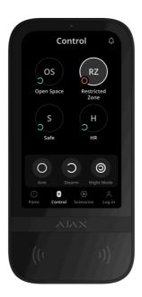
KeyPad TouchScreen allows controlling the groups' security (if **Group Mode** is enabled). You can also adjust the keypad **settings** to determine which groups will be shared (keypad groups). By default, all groups are visible on the keypad display in the **Control** • tab. You can learn more about group security management in **this section**.
