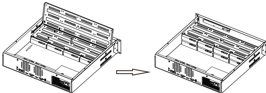
Step 5 Insert the hard disk data cable and power cable, then put on the upper cover and fasten the fixing screws.
