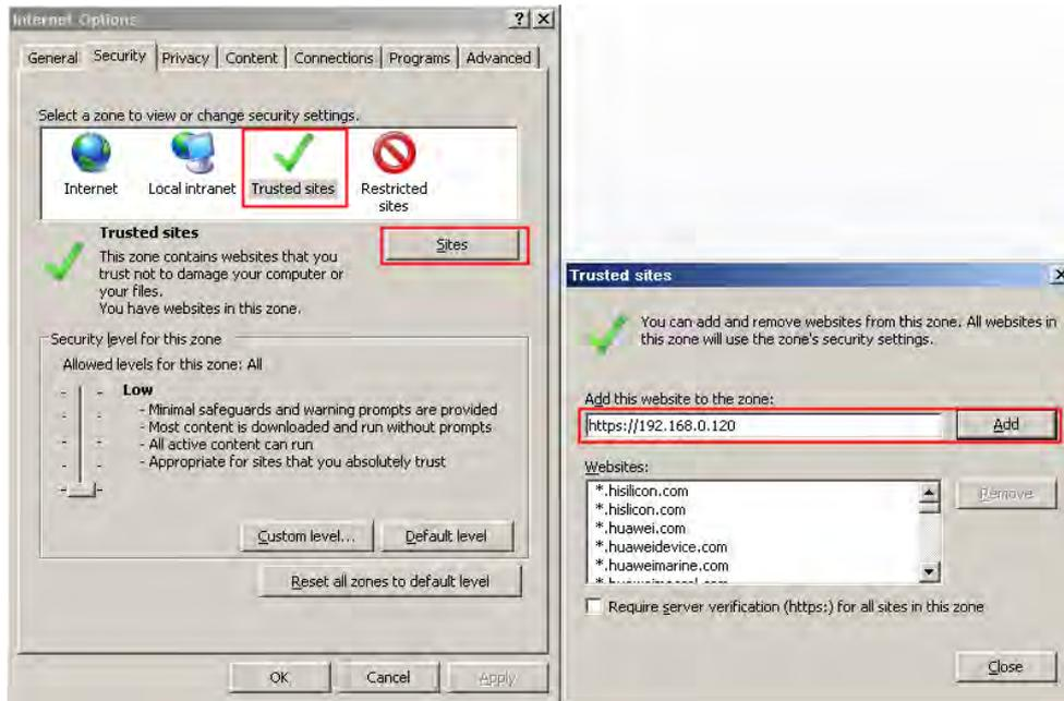
Step 2 In Internet Explorer, choose **Tools > Internet Options > Security > Customer level**, and set Download unsigned ActiveX controls and Initialize and script ActiveX controls not marked as safe for scripting under ActiveX controls and plug-ins to Enable, as shown in Figure 8-9.
