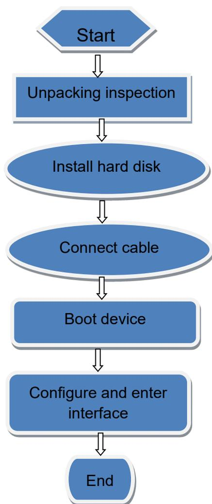
**Step 1** Check the appearance, packaging, and label of the device to ensure which no damage.
