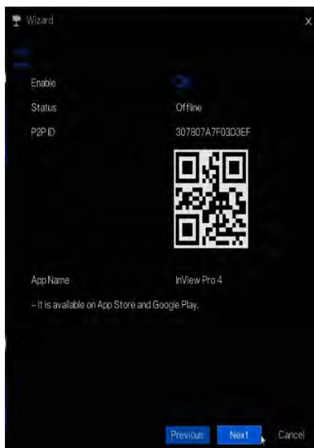
Step 8 When P2P is enabled, user can use mobile devices to manage the NVR by scanning the P2P ID, if the mobile phone has the RedVu GO app installed (search the APP at App Store or Google Play).
