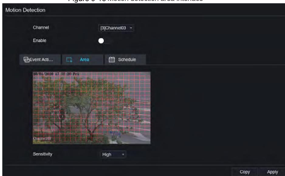
1. Hold down and drag the left mouse button to draw a motion detection area.
