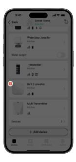
When the range extender detects a malfunction (for example, there is no external power supply), the Ajax app displays a badge with counter in the upper left corner of the device icon.
