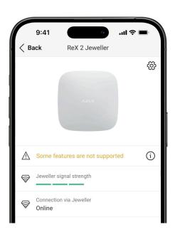
ReX 2 Jeweller can notify about malfunctions, if any. **Malfunctions** field is available in **Device States**. Clicking on (i) opens the list of all malfunctions. The field is displayed if a malfunction is detected.
