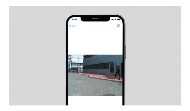
When the detector is triggered, the built-in MotionCam Outdoor camera can take 1 to 5 images with a resolution of  $320 \times 176$  and up to 3 images with a resolution of  $640 \times 352$  pixels. The detector has infrared illumination for shooting in the dark, which is activated only when an alarm is raised.
