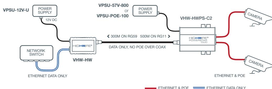
The diagram shows power injection at the Camera end, using a PSU for HIGHWIRE Powerstar Duo, with no power delivery
