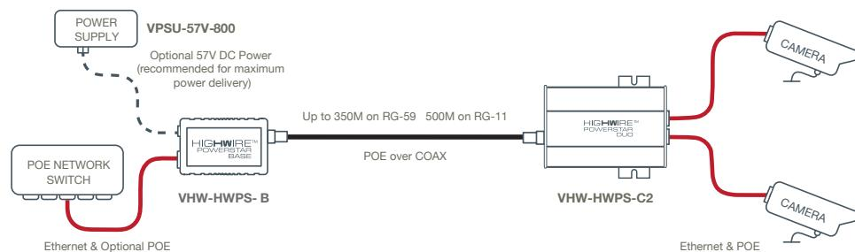
The diagram shows POE power delivery over coax from the Base end. The Powerstar Base unit may be powered by a POE or POE Plus switch, or for maximum power delivery
