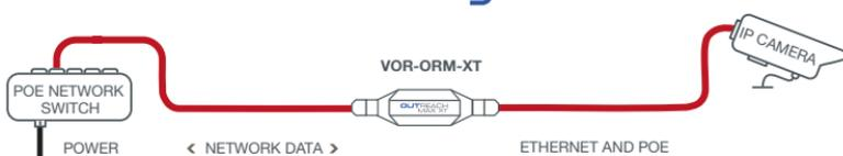
To extend Ethernet with POE, use OUTREACH Max XT to connect cable sections of up to 100 metres.
