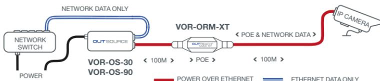
OUTSOURCE 30 and OUTSOURCE 90 are 802.3af/at/bt compliant injectors and may be connected to add or increase power for maximum power and range extension.
