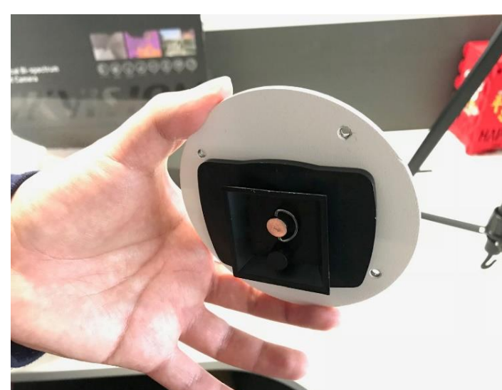
A. Tripod connector fixed on the adapter
