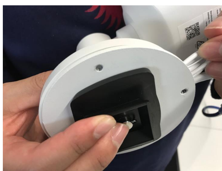
B. Fix the adapter on the camera
