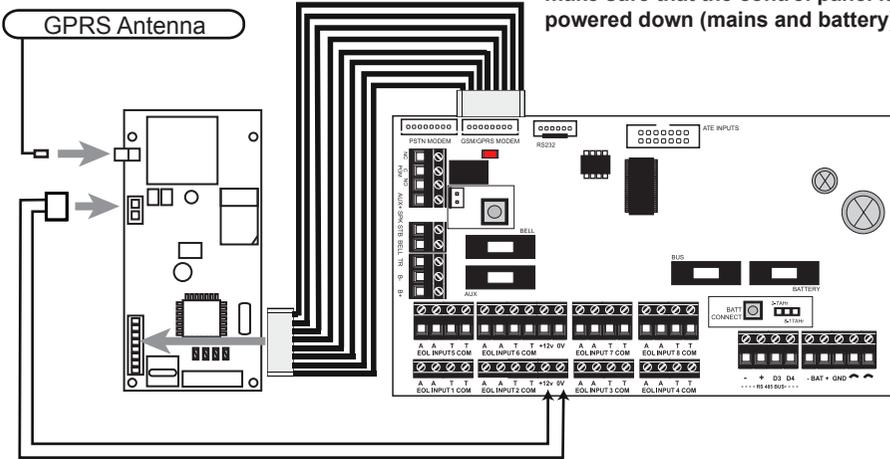
**NOTE:** When connecting a Digi GPRS to the Enforcer control panel, please use the power connector marked 'GSM modem' on the inside of the plastics.
